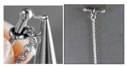
**Step 13** If wire ends create any rough spots, apply a small drop of Hypo Cement to the spot.
