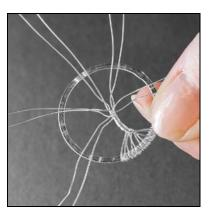
**Step 6**Begin twisting one pair of wires about halfway toward the component.
