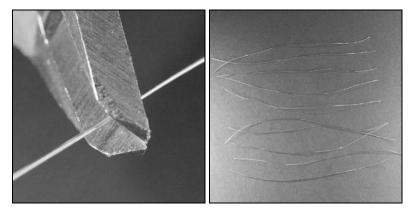
**Step 2**Anchor one length of wire to the component (see Covering a Component – Outer Edge Technique) by wrapping one end around the component three times. Trim the wire tail close to the component.
